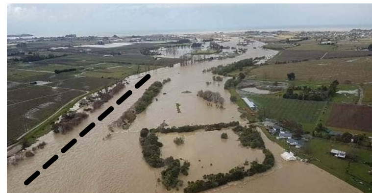
v The Motueka was well contained by stop banks. Note dotted line indicates normal channel.
