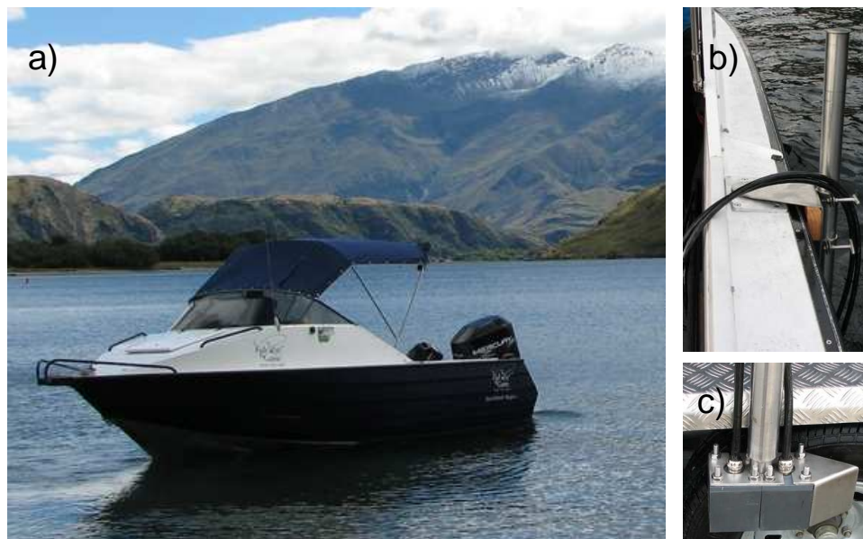
Figure 1: The New Zealand Fish and Game Southland Region vessel used for the survey (a), with the pole mounted amidships on the starboard gunwale (b), and the two transducers mounted at the end (c). The 200 kHz was not used in 2009.
