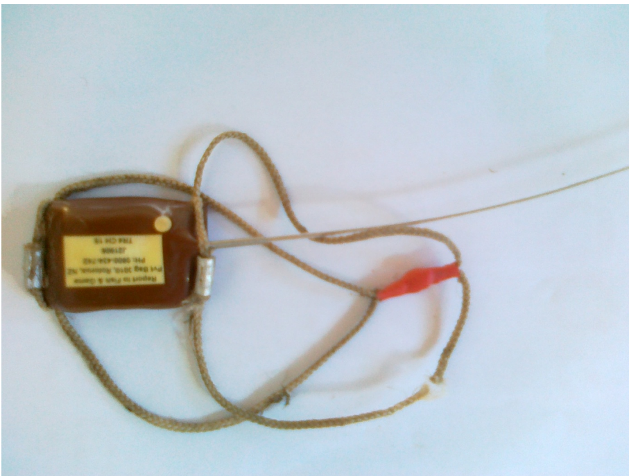
Figure 4. Backpack harness showing breastbone reef knot sheathed in red electrical heat shrink tubing
